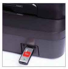
USB HUB FOR CONNECTION OF EXTERNAL DEVICES
